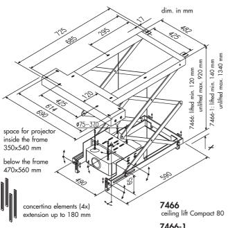
7466-1 projector weight max. 20 kg ceiling lift Compact 120 required ceiling cutout min. 600x500 mm
